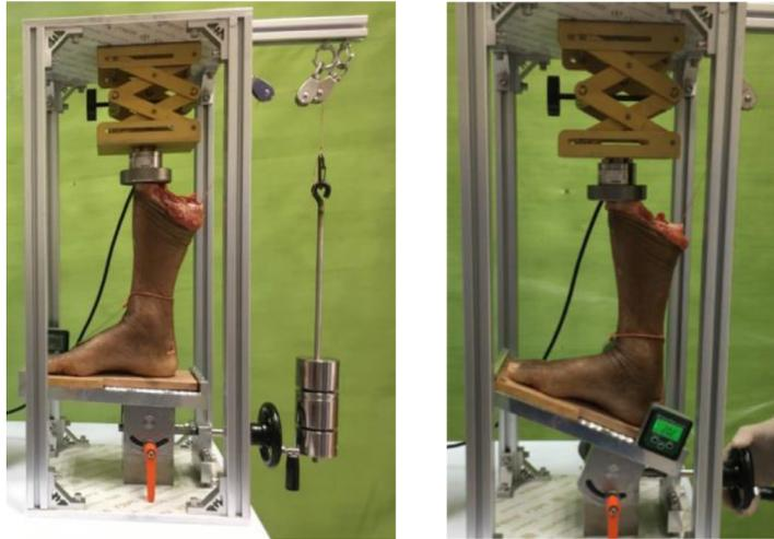
**Fig. 1.** Loading frame and setting of the cadaveric foot. The foot was set on the frame, and an axial load was applied to the tibia. The loading frame could control the sagittal kinematics of the ankle joint.
